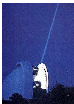
Fig. 2.4: Lunar laser ranging experiment laser
